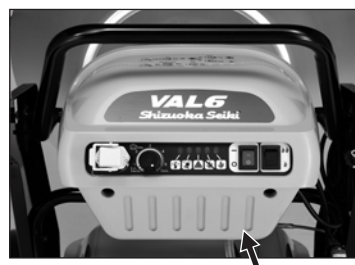
temperature sensor for Internal thermostat
