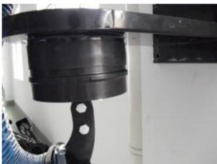
8. Tighten the PVC hose on the plastic flange with the hoop.
