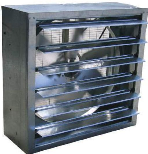
Primarily for use on large industrial sites or agricultural buildings, these fans are designed to move very large volumes of air. Manufactured from galvanised steel, these fans are built to last and come with automatic louvres which open and close according to operation. The Industrial Galvanised Louvred Fan can be used to exhaust heat, smoke, dust, or provide ventilation for livestock.
