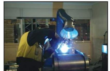
Welding & Fume Extractors are imperative for any workplace with welding and toxic fumes present.
