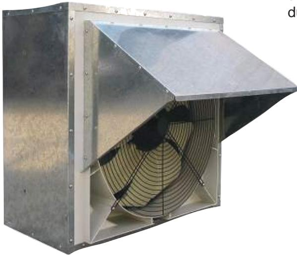
The Industrial Wall Exhaust Louvred fans are a 600mm axial wall fan predominantly used in larger buildings where generous airflow is required. These units extract at a rate of 5000 L/s come standard with internal gravity louvres and are made with a heavy duty construction. Comes with rain cover.
