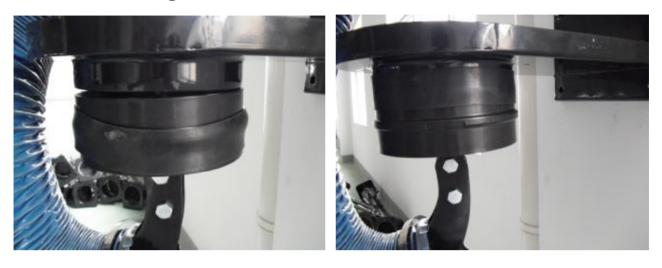
8. Tighten the PVC hose on the plastic flange with the hoop.
