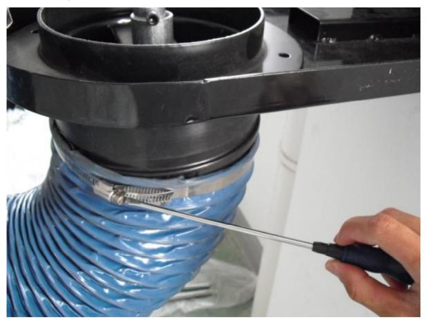
9. Tighten the PVC hose on the hood with the hoop.
