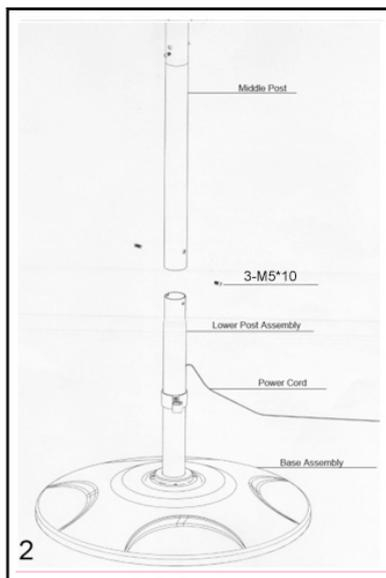
Secure that the lower post assembly (11) and the middle post (9) using 3 x M5 X 10 screws
