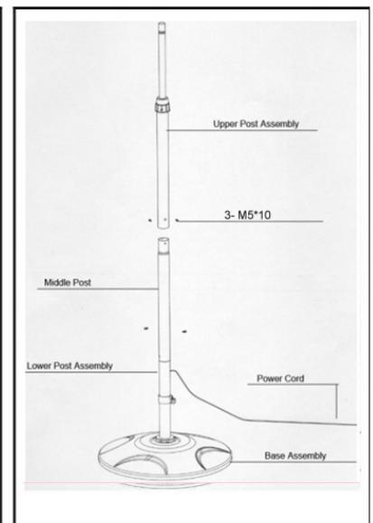
Secure the upper post assembly (7) and the middle post (9) using 3x M5 X 10 screws (fig.3)
