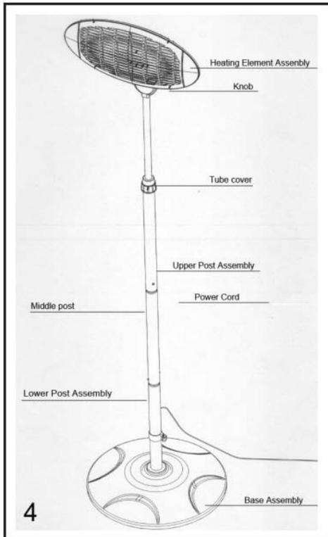
Attach the heating element (1) to the upper post assembly (7) and secure it by tightening the button (fig.4)
