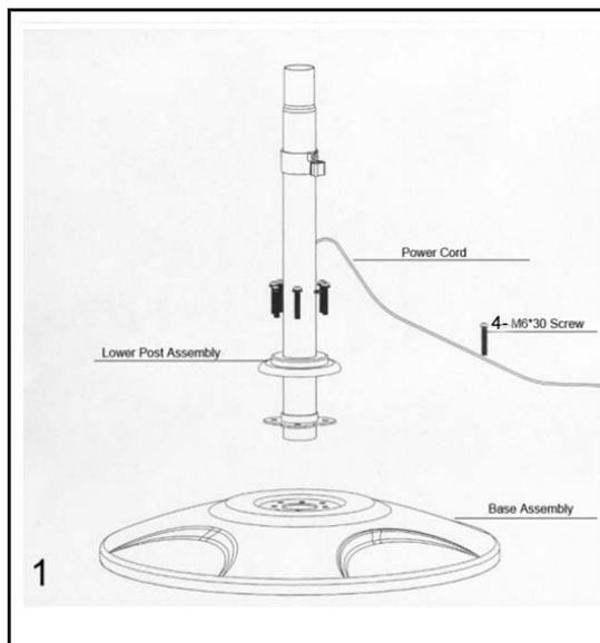
Insert the lower post assembly (11) into the foot plate/base (15) and secure it using 4x M6 X 30 screws (fig.1)
